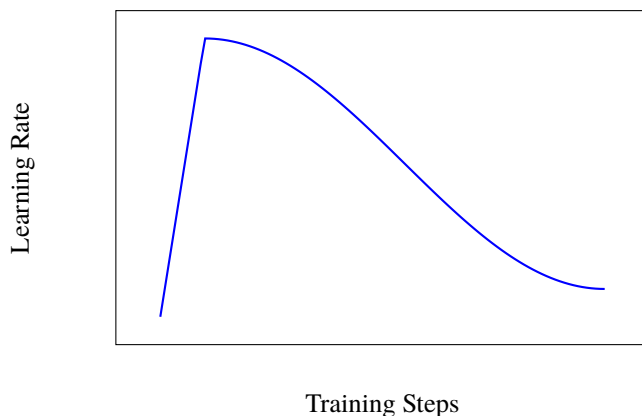
Figure 2.5: Example of a learning rate schedule combining warmup (first 10 steps) and cosine decay (remaining steps)
